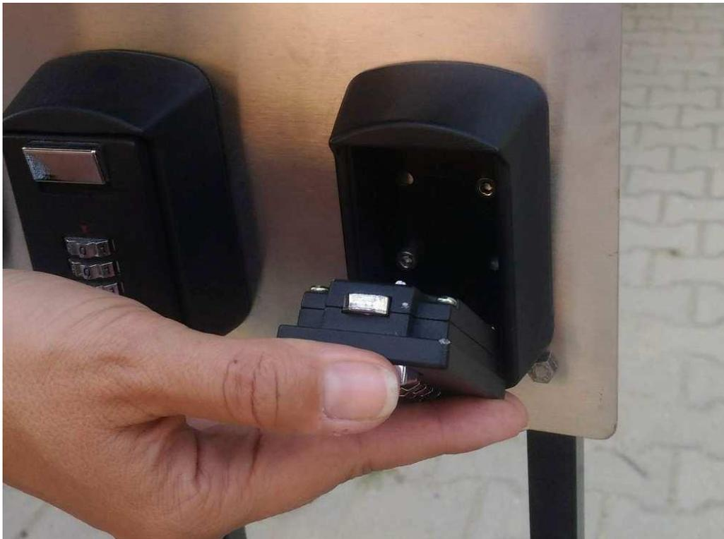
To replace the box lid, reverse the procedure. Attach the lower part of lid, in the upper part you can help with press of silver rectangular button. A clear click should be heard after contact.
